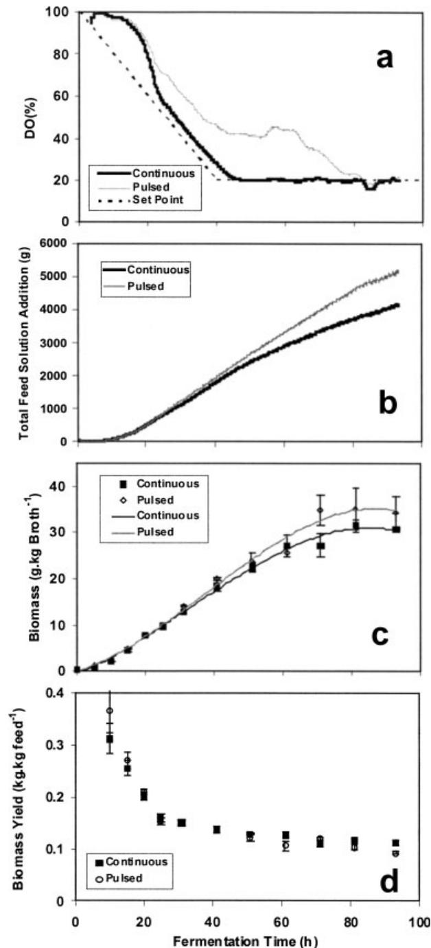
**Figure 1.** Results from three pulsed and three continuously fed *A. oryzae* fermentations, operated in 20-L fermentors. (a) Dissolved oxygen (DO) set-point and profiles, (b) average biomass concentration, (c) total carbon feed solution added, and (d) biomass yield factor, vs. time. In (b) and (d), error bars represent standard error and lines drawn in to illustrate trends. Each line in (a) and (c) represents the average of three fermentations.
