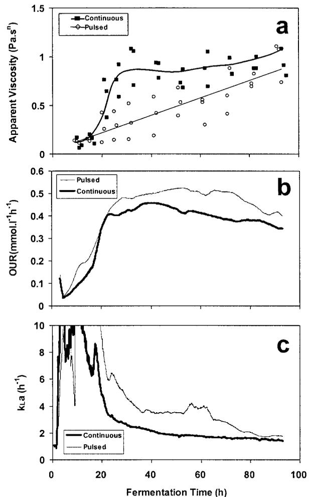
**Figure 3.** (a) Apparent viscosity (at a shear rate =  $20 \text{ s}^{-1}$ ), (b) oxygen-uptake rate (OUR), and (c) oxygen mass-transfer coefficient ( $k_La$ ) for the three pulse-fed and three continuously fed fermentations described here. Lines drawn in (a) illustrate trends, those in (b) and (c) represent average values.
