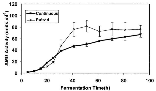
**Figure 2.** Product (glucoamylase) activity profile for three pulse-fed and three continuously fed fermentations. Error bars represent standard error.
